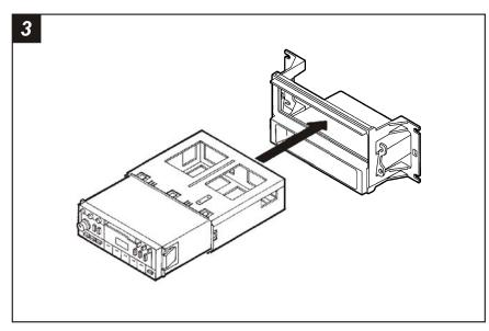
Slide the DIN cage into the Radio Housing and secure by bending the metal locking tabs down. Slide the aftermarket head unit into the cage until secure.
