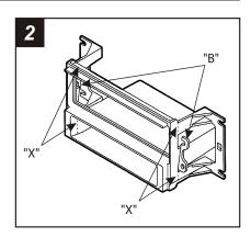
Locate tabs "B" on the Radio Housing. and remove the mounting legs containing tabs "A" by cutting along dotted lines "X". Skip to the Installation Instructions for ALL VEHICLES on Page #2.
