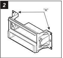
Locate tabs "A" on the Radio Housing. Skip to the Installation Instructions for ALL VEHICLES on Page #2.
