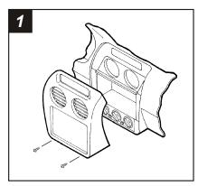
Disconnect the negative battery terminal to prevent an accidental short circuit. Remove (2) Phillips screws under the climate controls. Unclip the radio/climate control trim bezel and remove the bezel. Remove (4) Phillips securing the factory head unit and disconnect the wiring.
