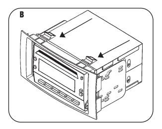
Note: This installation kit is an extremely tight fit and requires force to be "snapped" into the dash opening. Removal of aftermarket radio is even more difficult than installation, so please be sure to fully test the aftermarket radio prior to completeing the kit's installation.
