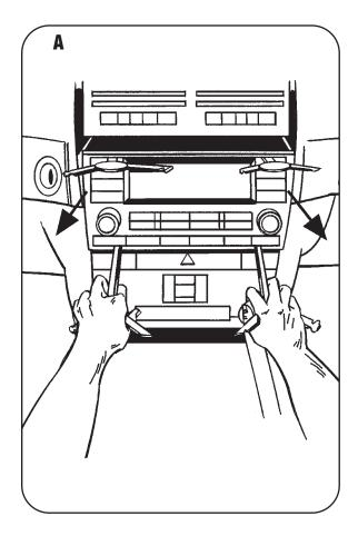
Note: This installation kit is an extremely tight fit and requires force to be "snapped" into the dash opening. Removal of aftermarket radio is even more difficult than installation, so please be sure to fully test the aftermarket radio prior to completeing the kit's installation.
