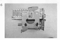
Remove the original mounting bracket. This is tighten by eight screws.
