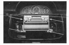
Remove the original radio. The radio is tighten by four screws.
